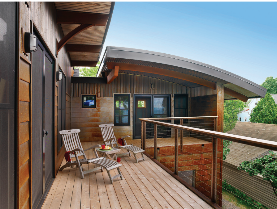
The home's deck offers a panoramic view of Lake Champlain and the Adirondacks. It includes curved structural beams and Cor-Ten siding that rusted to a dark patina. The rear of the structure is in sharp contrast to the home's front exterior, which was mandated to remain compliant with the character of the downtown Burlington neighborhood.
